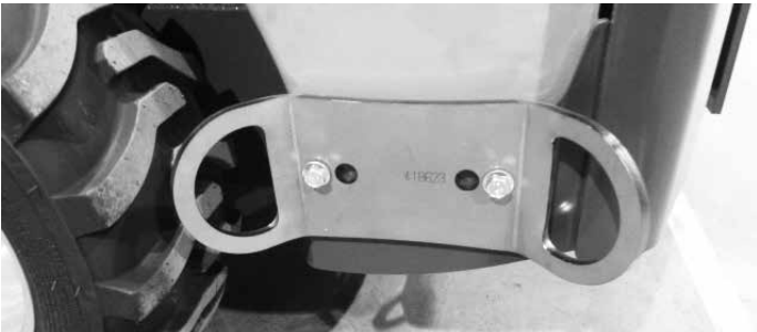
Tie down bracket A418623 installed at the side of rear frame. For side installation, two brackets are needed.
