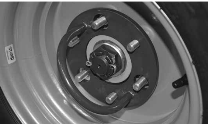
Tie down bracket on wheel hub A423161
